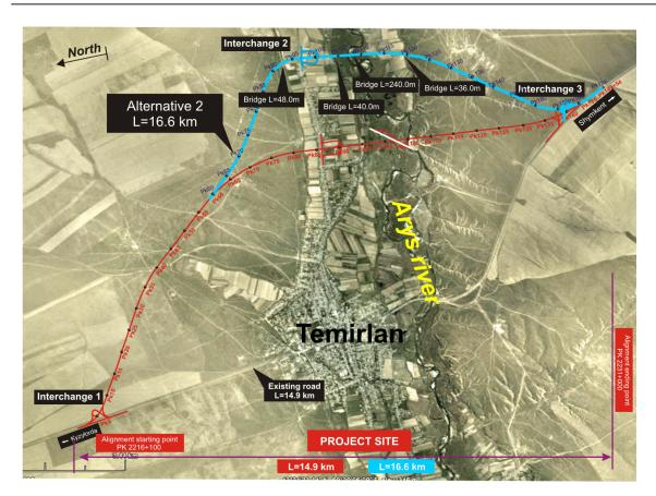
Figure 7.1 Alignment Alternatives.
